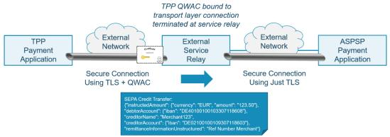
Figure B-3: Illustration of Transaction Passed Through External Service Relay
