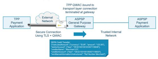
Figure B-2: Illustration of Transaction Passing Through ASPSP Gateway
