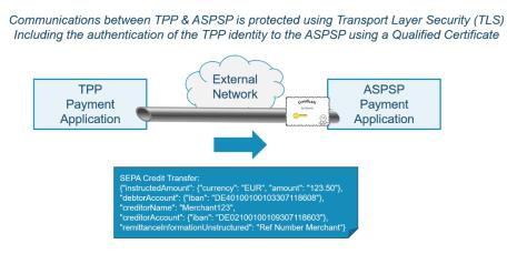
Figure B-1: Illustration of End to End Transport Layer Security
